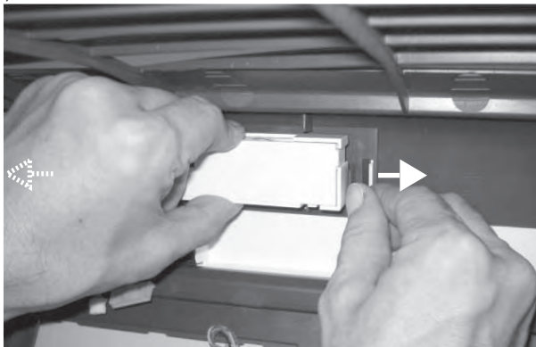
16)The display assembly is removed. (right and left two hooks place)
