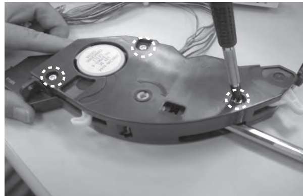
20)The panel mechanism cover is removed. (3 screws)
