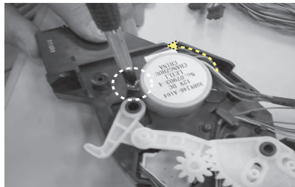
21)The screw that is the fixation of the panel motor is removed, and is turned to the left and it is removed.
